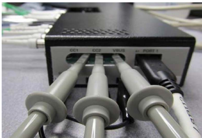
Figure 10. VBus probing on N7018A
